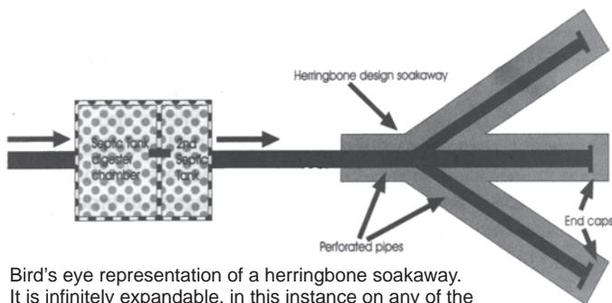
Bird's eye representation of a herringbone soakaway. It is infinitely expandable, in this instance on any of the three arms, so long as sufficient fall is maintained.
